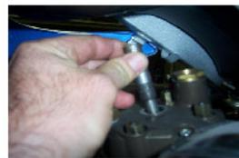
RETIRER LE BLOQUE PISTON ET REPOSITIONNER LA BOUGIE AVEC SON ANTI PARASITE.
