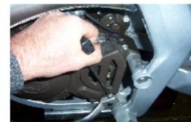
REPOSITIONNER AVEC UNE CLÉ A PIPE DE 10 LA VIS DE FIXATION DU SÉLECTEUR.
