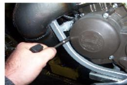
REPOSITIONNER LES 3 VIS DE FIXATION DU CARTER D'ALLUMAGE AVEC UNE CLÉ A PIPE DE 8.
